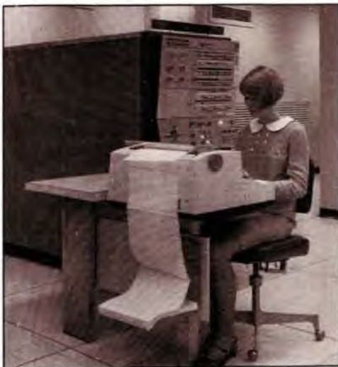
The first computer centre was opened by the Department in 1967. Shown is the display panel and console typewriter of the IBM 360/40 in the New South Wales State Headquarters.
